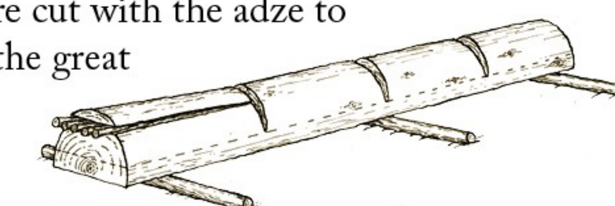
Sketch showing the manufacturing of boards and planks. Illustration by Louis Shotridge, in The Museum Journal 4:3-90 (1913), University of Pennsylvania.
